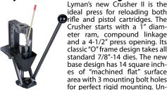
ideal press for reloading both rifle and pistol cartridges. The Crusher starts with a 1" diameter ram, compound linkage and a 4-1/2" press opening. Its classic "O" frame design takes all standard 7/8"-14 dies. The new base design has 14 square inches of "machined flat" surface area with 3 mounting bolt holes for perfect rigid mounting. Un-
